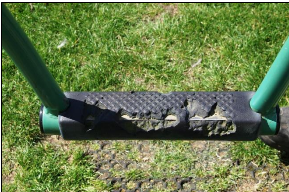
Fig. 7: Damaged tread on Rocker.
