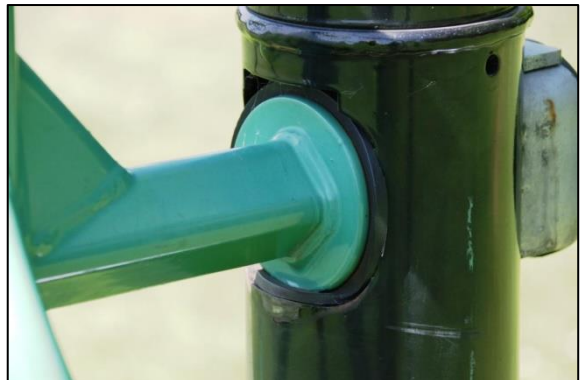
Fig. 8: Worn bush on Rocker.
